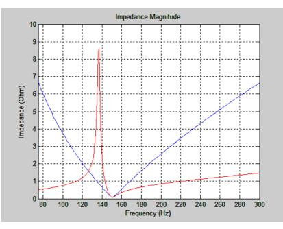
In some cases of wrong design or due to ageing of filter equipment, the latter especially causing a capacitance drop, the parallel resonance frequency changes in such a way that it may coincide with a current harmonic frequency injected by the load. This will cause overvoltages and overcurrents in the system equipment, leading to failure; and in some cases together with catastrophic damage.
